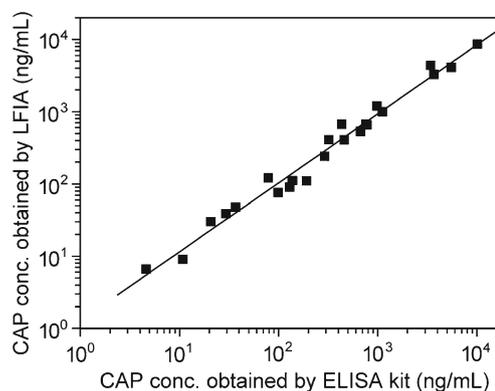
**Fig. 3** Correlation between commercial CAP ELISA kit and Eu(III) CAP nanoparticle-based LFIA for quantification of 23 CAP positive cow milk samples ( $r^2=0.9803$ ,  $P<0.0001$ ,  $n=23$ )
