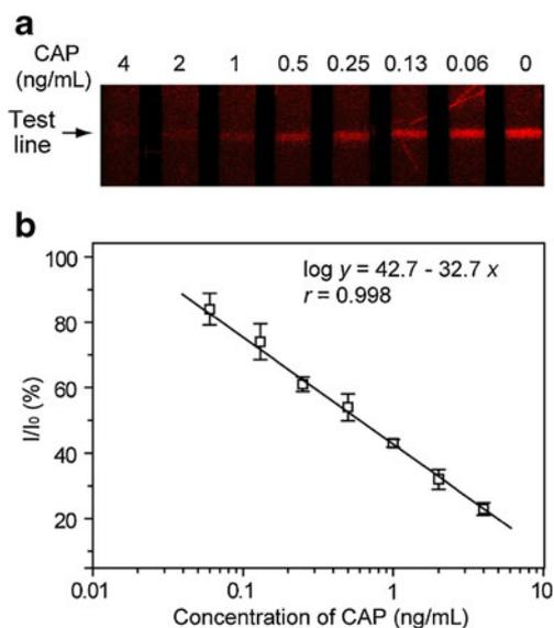
**Fig. 2** Eu(III) nanoparticle-based LFIA of CAP standards. **a** Digital image of test strips (membrane area) carried out with 2-fold serially diluted CAP standards and a negative control in assay buffer; **b** calibration line obtained from panel (a). At each concentration point, the error bar indicates the SD from six independent measurements
