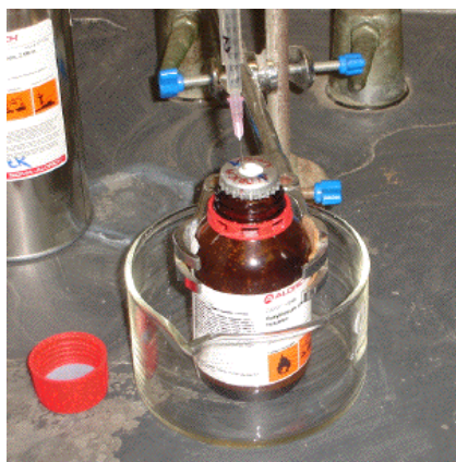
Image 1: Restraint of reagent bottle prior to use and introduction of inert gas input line.
