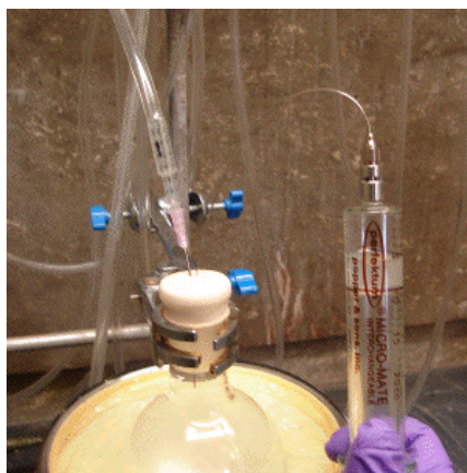
Image 7: Puncture of reaction vessel septum and displacement of inert gas cushion above reagent.
