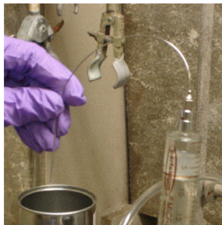
Image 6: Transport of the pyrophoric reagent to the reaction vessel while under a protective cushion of inert gas within the inverted syringe.
