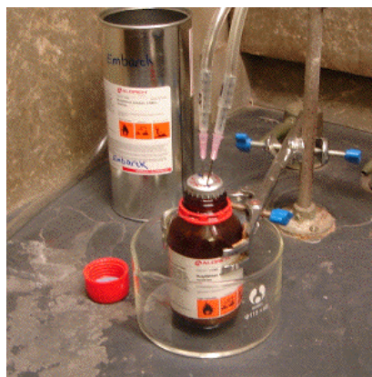
Image 2: Purging the reagent bottle with inert gas; the tube on the left is an input flow of Ar, while that on the right is a bubbler terminated output line.
