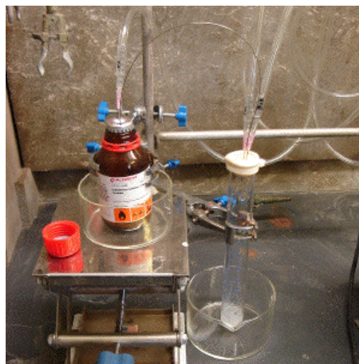
Image 10: Transfer of reagent into measuring cylinder. Note bubbler terminated output line on the receiving vessel; at this stage, the inert gas input line into the reagent bottle is open, but that into the receiving flask is closed.
