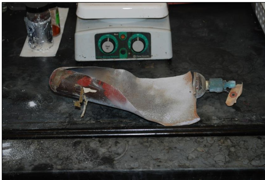
Figure 14.2 – HF Cylinder Incident at University of Michigan in 2011
